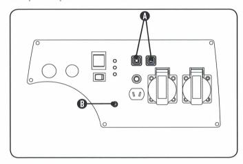
6. Plug the other pair of power leads (A), and ground wire (B) to inverter #2.
